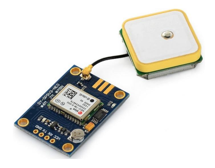
• This module has an external antenna and built-in EEPROM.
